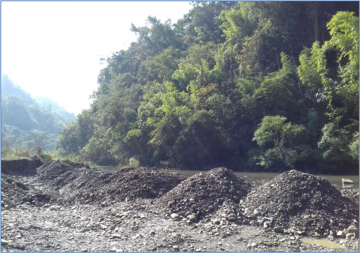
Fig.1: Granular Sub Base deposited at Tuipui River
