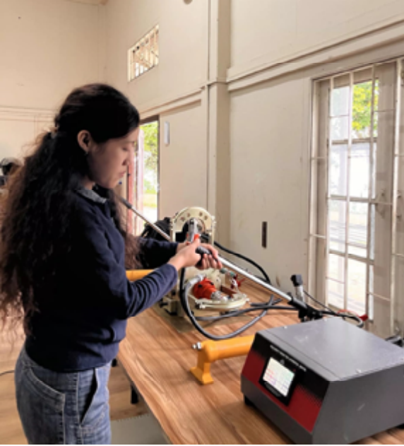
Rock direct shear test apparatus
